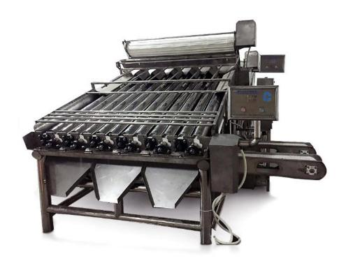
The main part of our shrimp grading machine is made by SUS304 stainless steel, correspond to food hygiene requirements. The machine is consisted of two parts: elevating and grading unit, grading unit has 4-6 couples of roller which shape is up-thick and bottom-thin. The shrimp is graded by the gap between two rollers automatically. The gap is available to adjust. There are 5 graders are under controlling. Accuracy of shrimp size reach to 0.1mm.
