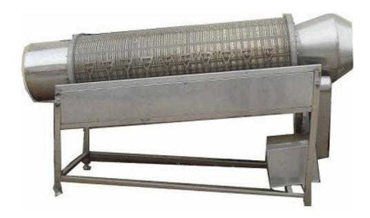
This machine is designed to cut or 'snip' the ends from string beans. It has a high capacity and flexibility and provides a gentle product treatment. The bean snipper is easy to clean, and up to the high hygiene standard.
